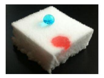
Nanocellulose sponges for oil remediation are another example of the vast range of applications offered by nanocellulose. Developed at EMPA - the Swiss Federal Laboratories for Materials Science & Technology - the sponges absorb great quantities of oil while floating on water. The hydrophobic sponges consist of silylated nanocellulose. They can be made from pulp, straw or recycled paper. **Read more**
