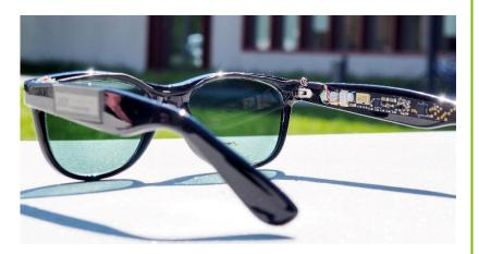
Organic solar cells are flexible, transparent, and light-weight – and can be manufactured in arbitrary shapes or colors. Thus, they are suitable for a variety of applications that cannot be realized with conventional silicon solar cells.
