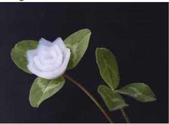
EMPA researchers have succeeded in producing 3D printed parts from silica aerogel with high precision. This opens up numerous new applications in the high-tech industry, for example in microelectronics, robotics, biotechnology and sensor technology.
