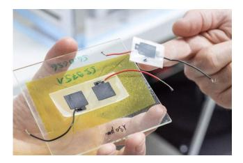
The number of data-transmitting microdevices, for instance in packaging and transport logistics, will increase sharply in the coming years. All these devices need energy, but the amount of batteries would have a major impact on the environment. Empa researchers have developed a biodegradable minicapacitor that can solve the problem. It consists of carbon, cellulose, glycerin and table salt. And it works reliably.
